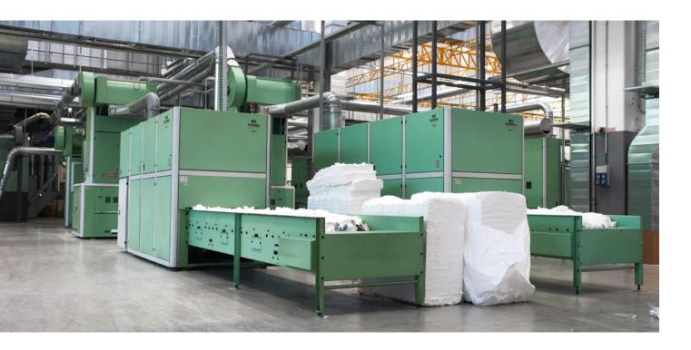
Industry experts argue that blow room and carding machinery used in the spinning preparation process entail substantial advantages for nonwoven producers working in the hygiene and medical sectors.
