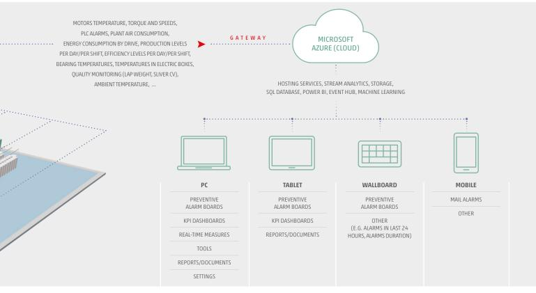
The client can always access the dedicated portal where it is possible to see the information for predictive maintenance of the machines and of the overall efficiency of the plant.
