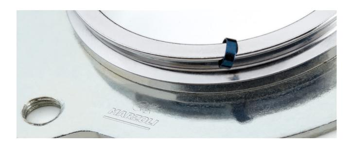
Few components on the ring spinning frame are as important as the ring. The ring without doubt is the component that, along with the ring traveler, mostly affect the spinning frame productivity and the end-product quality. In order to ensure that the client with a Marzoli spinning frame relies on the mostly advanced and reliable technology, Marzoli has decided to draw on its superior competence and expertise to develop its own-branded ring.
