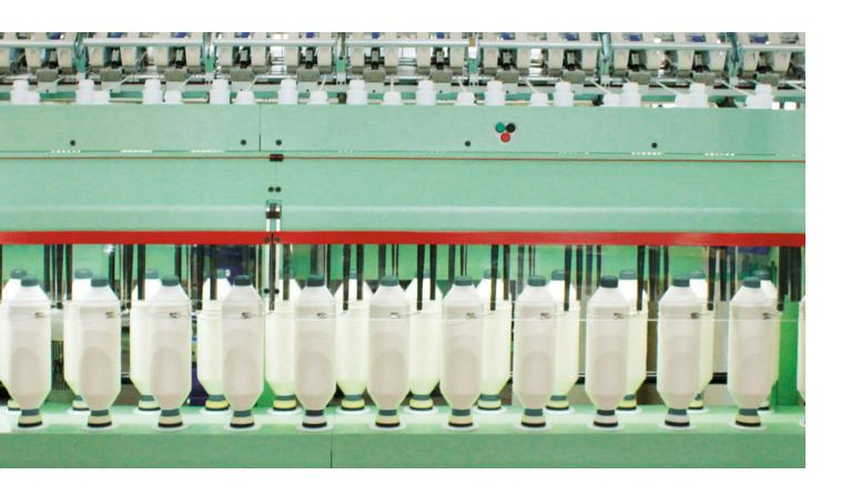
The Marzoli R<sup>2</sup>S system with statistics for roving break detection controls each spindle using a reflective photocell which constantly monitors the presence of the roving, promptly signalling any breakage by means of serial communication to the control board, which immediately sends a stop signal to the bench along with the number of the broken roving.
