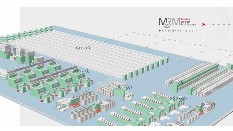
MRM is an innovative software platform developed by Marzoli that continuously analyzes the symptomatic data gathered by processors and sensors installed in critical parts of the machines to constantly monitor their efficiency. The data about temperatures, power consumption, pressures, speeds and vibrations are gathered and, through a gateway, are sent to the Azure Cloud provided by Microsoft.
